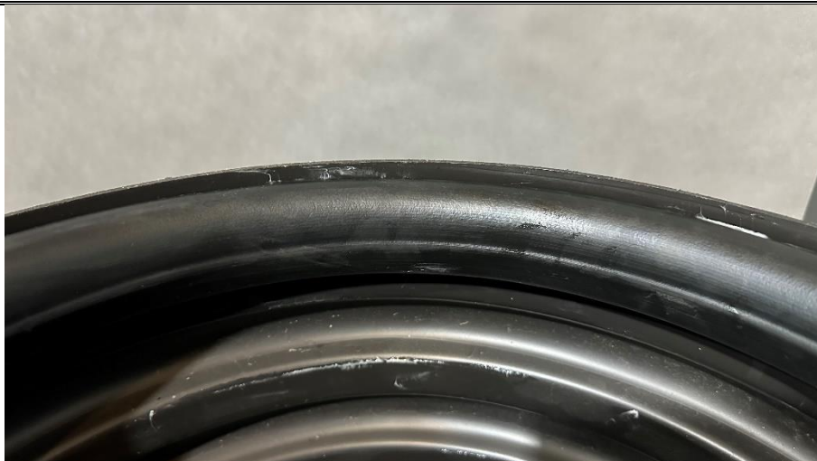
Fig.5 – installation of the gasket in the pipe valley (depending on the pipe, the gasket may be positioned differently).
