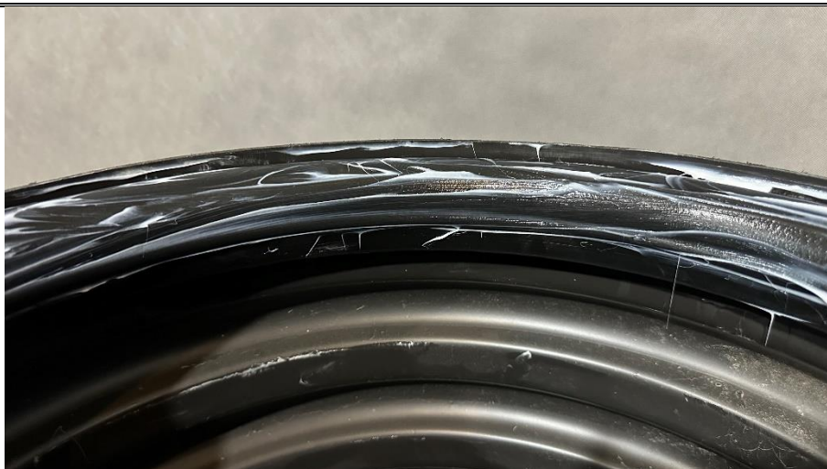
Fig.6 - Implementation of lubricant on the seal for correct plug installation - T4/600/Z.
