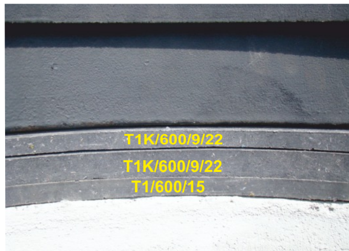
Standard application of TVR T System rings in concrete finial structures as the element adjusting the sitting height of manhole and damper. Plastic compensation rings with height of 15, 30, and 40 mm and T1K/600/9/22 or T1K/625/9/22 and T1K/635/30/60mm wedge rings eliminate the use of unreliable cement mortars.
