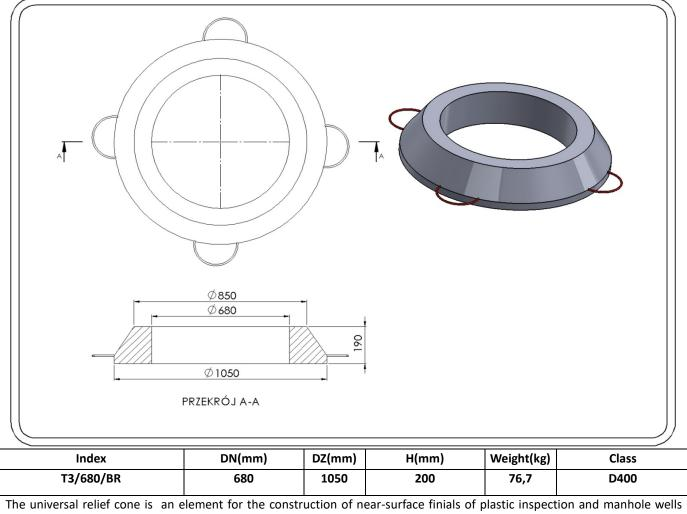
DN/ID 600 and DN/OD max 675mm in class D400. The T3/680/ BR relief cone enables full relief / protection of the shaft of the rising pipe of the plastic chamber against traffic loads. It provides direct support for manholes acc. to DIN 19584 (BEGU type), self-leveling manholes with the outer diameter of the leading pipe 665  $\div$  675 (KZO DN600, Viatop Niveau), compensation
